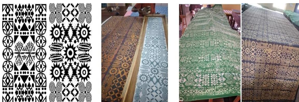
Fig. 1: Designed artwork, Discharge screen printing and Finished discharge printed Fabrics (Field study, 2021)
